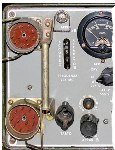
Front panel photo cutout of an Italian Army refurbished Wireless Set Canadian No. 19 Mk.III showing the 'B' set section.
